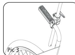
Thanks to the linkage with the two articulated joints, the fastening unit of the model MT-IN-SCHV22 (pic. 4) can be mounted on almost any suitable tube in the frame (pic. 5 and 6). Thanks to the articulated joints, it can be adjusted individually. The linkage can be detached from the fastening unit at any time by loosening the quick release and thus dismantled, while the fastening unit remains on the wheelchair.
